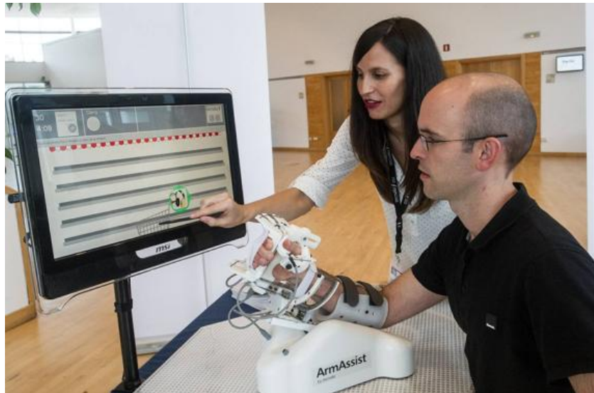
Figure 4: Example of a robot for rehabilitation of upper limb in patients who have suffered stroke (Source: Tecnalia)
