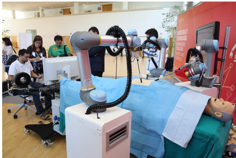
Figure 3: Example of tele operated robotic system for laparoscopic surgery (Source: Tecnia)
