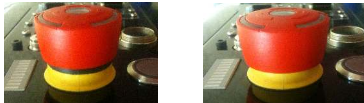
Figure 34: Emergency button in normal state (left), emergency button in pressed state (right)
