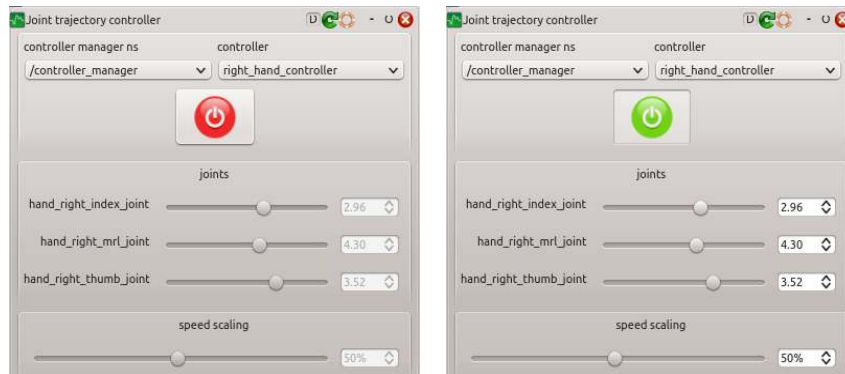
Figure 117: Detail of the joint control panel in monitor (left) and control (right) modes.
