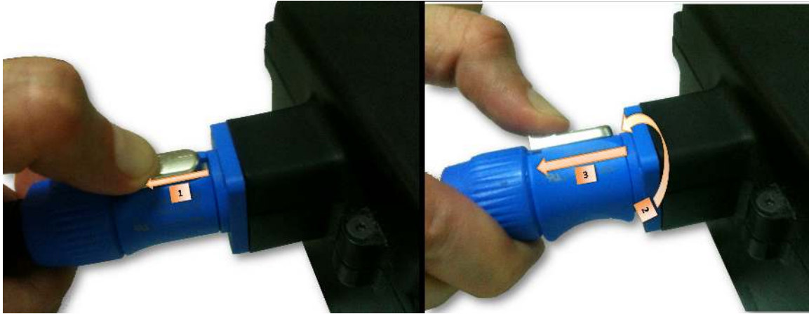
Figure 38: Unplugging charger
