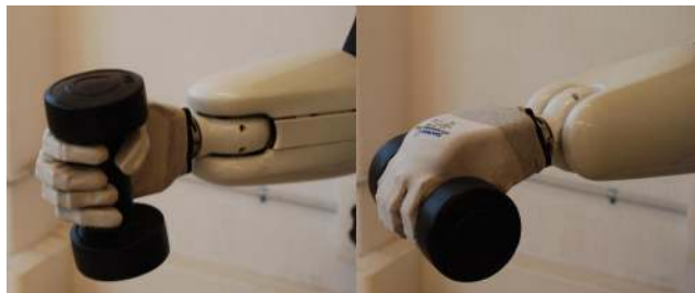
Figure 127: Dumbbell being grasped at different hand orientations.
