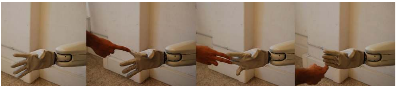
Figure 123: External disturbances applied to hand with slack finger tendons. From left to right: Open hand, index hyperextension, middle and ring hyperextension, abduction disturbance.
