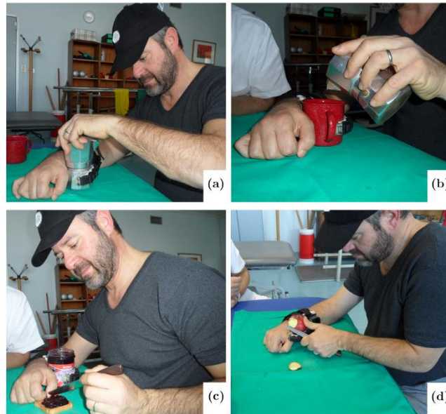
PICTURE IRSIPAA 10 THE ROBOTIC SIXTH FINGER USED BY A PATIENT IN SOME ACTIVITIES OF DAILY LIVING
