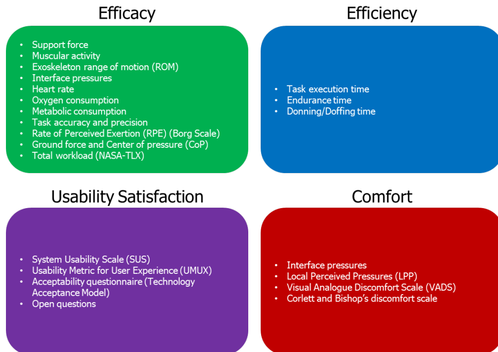
Figure 10: Exoskeleton parameters classified according to efficacy, efficiency, usability satisfaction and comfort
