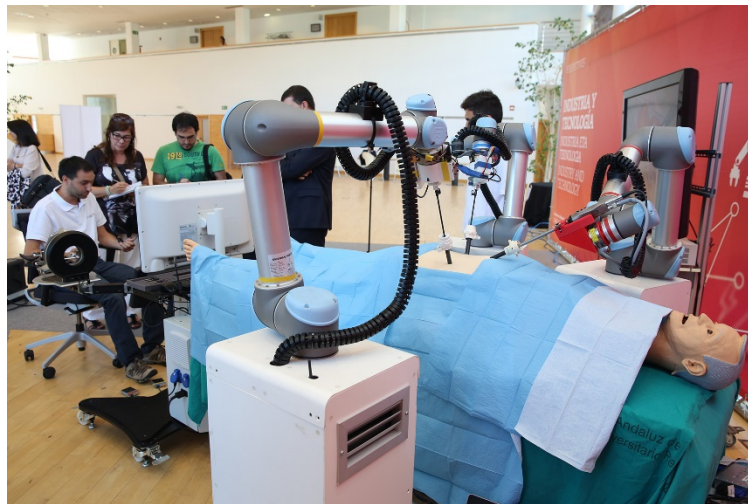
Figure 3: Example of tele operated robotic system for laparoscopic surgery (Source: Tecnalia)
