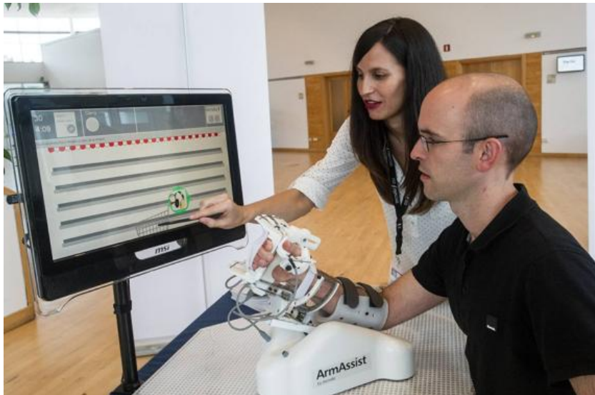
Figure 4: Example of a robot for rehabilitation of upper limb in patients who have suffered stroke (Source: Tecnia)
